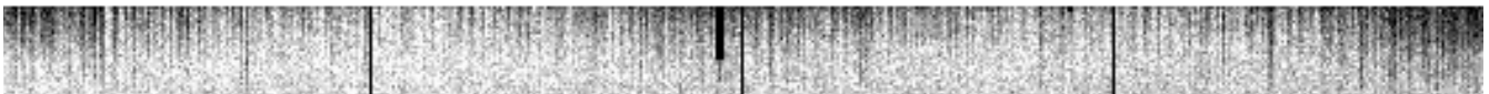
Fig. 1— Image of the S3 chip in the Mn line. The image was blocked by a factor of 16 along the CHIPY direction to emphasize the column-to-column variations
